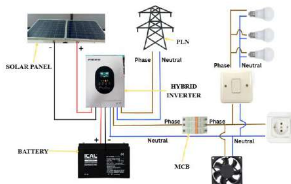
Figure 5. Design of the hybrid solar power system
