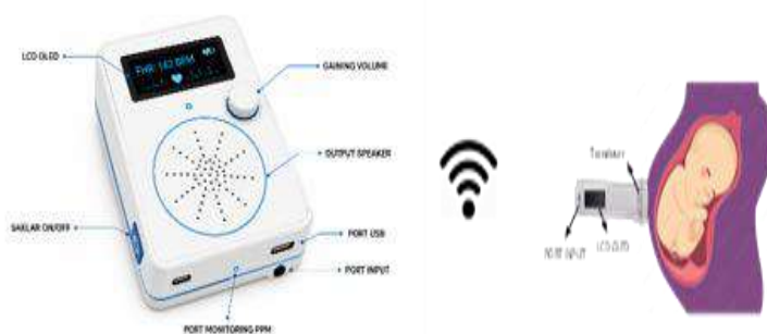
Figure 1. Implementation of fetal heart rate (FHR) monitoring using a wireless fetal doppler with FHR sound enhancement and digital filter for noise reduction
