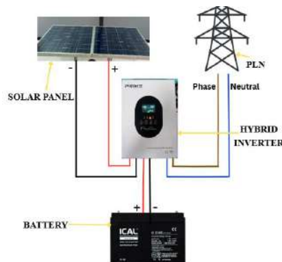
Figure 3. Configuration of the proposed hybrid solar power system
