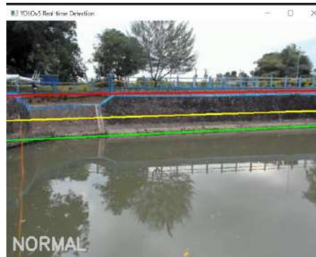
Figure 3. ROI-based water level monitoring strategy
