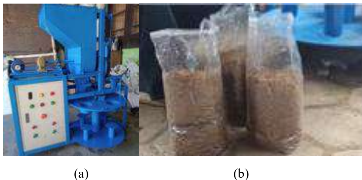
Figure 5. Oyster mushroom mixer machine prototype
