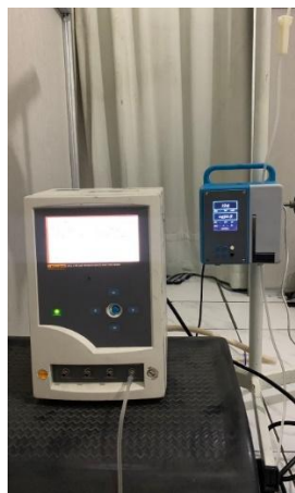
Figure 12. Documentation of Flow rate data collection process using IDA
