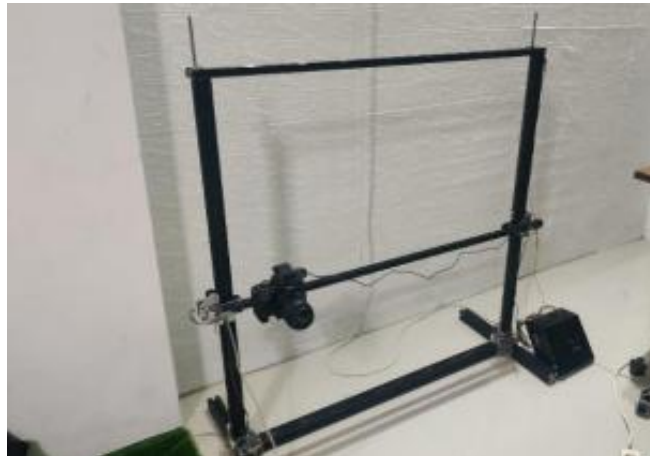
Figure 4 Mechanical of the Automatic Camera System
