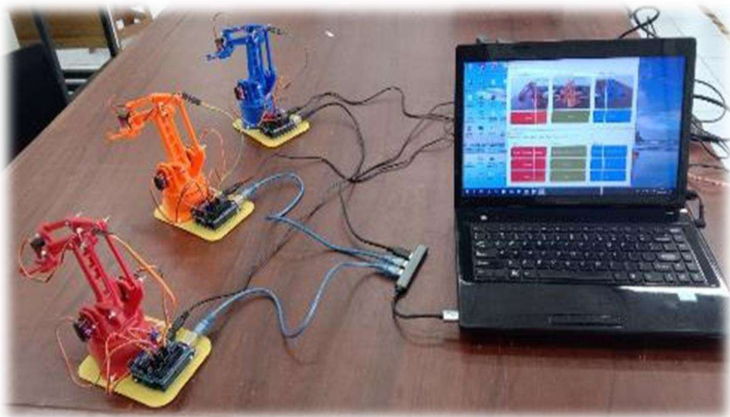
Figure 6. Experimental setup of the 4-DoF multi-robot arm.
