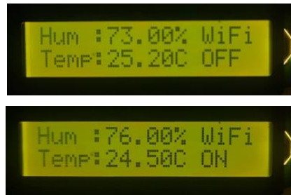
Figure 5. LCD screen display on mushroom cultivation house to display sensor readings and WiFi connection status
