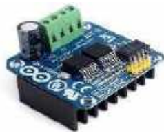
Gambar 2. Driver Motor BTS7960
