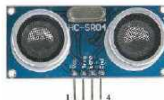
Gambar 2. Sensor Ultrasonik HC-SR04
