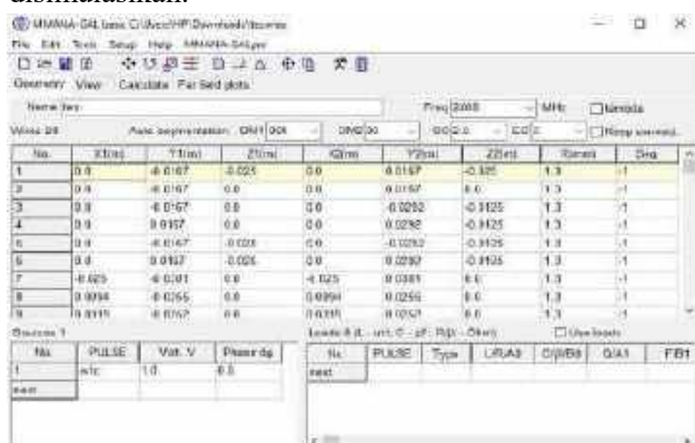
Gambar 12. Geometry antena Yagi penerima 2400MHz
