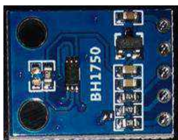
Gambar 3. Sensor Intensitas Cahaya BH1750
