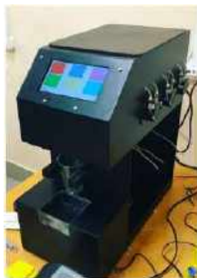
Gambar 3. Smart bartender with peristaltic pumps
