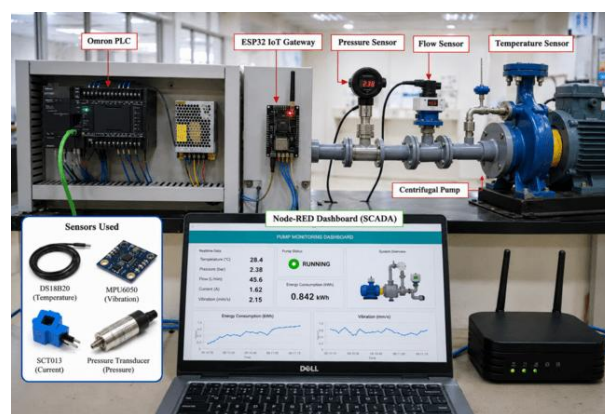
Figure 3. Experimental setup of the proposed adaptive PLC-SCADA system
