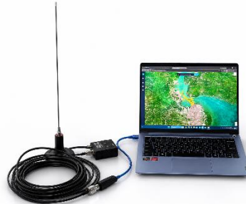
Figure 3. Hardware implementation of the AIS receiver system
