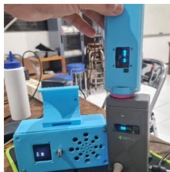
Figure 5. Measurement results with different bpm settings using fetal simulator
