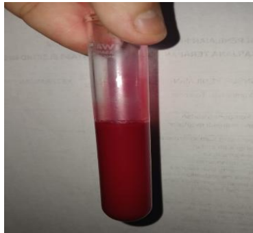
Figure 4. Sample separation result using PWM control (TON = 5.8%, 30 minutes)
