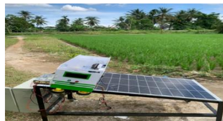
Figure 7. Testing and measuring solar panels after cleaned up
