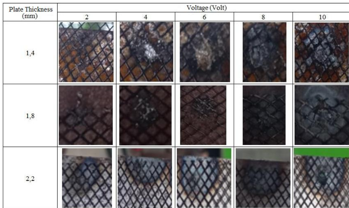
Figure 7. Spot Welding Test
