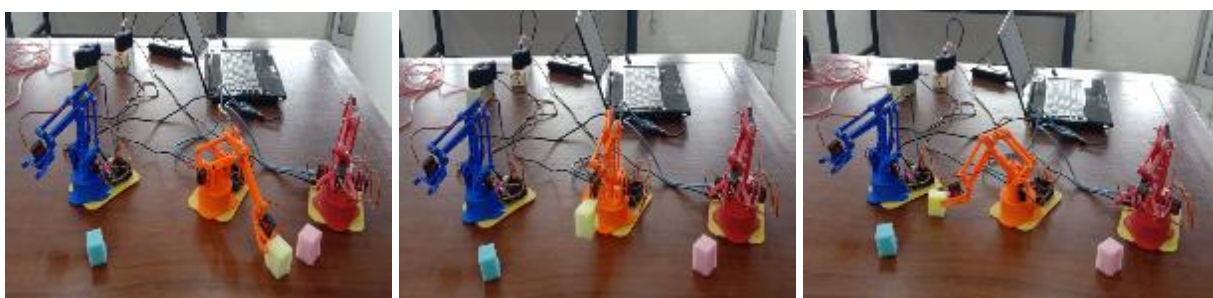
Figure 11. The movement of the orange robot in picking up objects, (a) the robot picks up an object, (b) moves the object, and (c) places and releases the object
