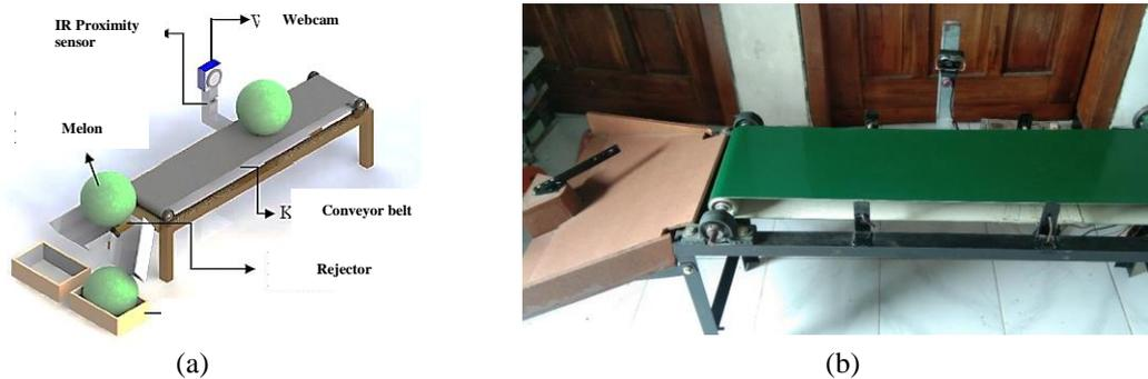
**Figure 3.** (a) Sorting Mechanism 3D Design (b) Design Realization
