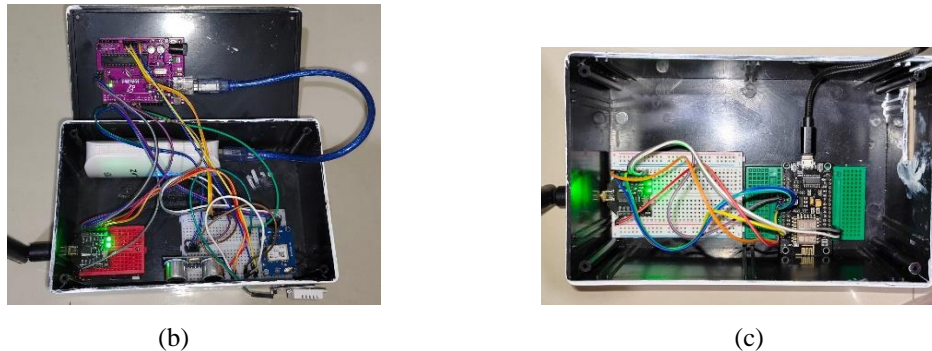
Figure 7. (a) Waste management system prototype, (b) The interior of end node, (c) The interior of gateway
