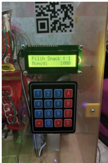
Figure 10. Keypad Test and QR Code Scan
